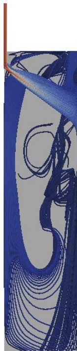
Steel flow inside the slab without EMBr - CFD Simulation
