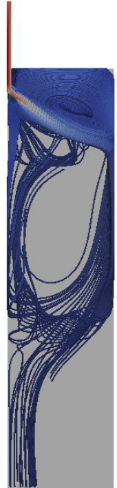
Steel flow inside the slab with EMBr - CFD Simulation
